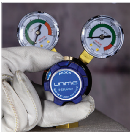
(6) Carefully open the valve of the gas cylinder, set the flow to 6-10 l/min
